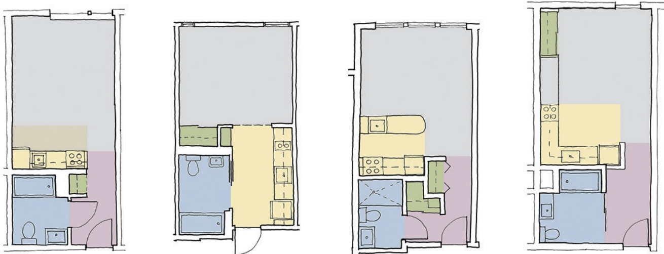
Figure 1. Kitchen Location Typology (l to r): Main room at Urness (with kitchen overlapping living area); Entry at Richardson; Separate galley at Dunbar; Separate L-style at The Six.
